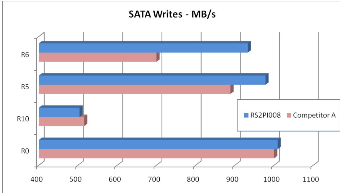
Figure 1. Competitive performance analysis for controllers with 24 3Gb/s 7200 RPM SATA hard drives in write-intensive environments
